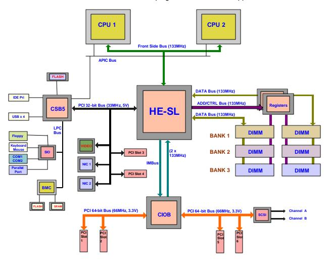
Figure 1. SDS2 Server Board Block Diagram
